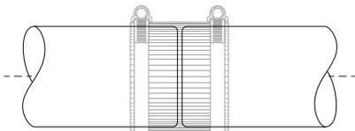
**1. TRANSFERENCE OF TORQUE:** Thicker gauge shield material "blocks" the torque from getting to the gasket. A thinner shield protects the gasket while allowing a more efficient transfer of torque therefore providing a better seal.
